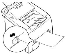
**Note**: When printing on previously printed paper from the manual feeder, the printed side should be facing down with an uncurled edge to the machine. If you experience problems with paper feed, turn the paper around.
